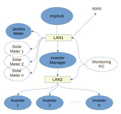
For LAN2 to the Inverter Manager assigns IP addresses using DHCP. For LAN1 the devices should be on fixed IPs, either statically assigned or DHCP reserved. In advance of the install, you will need to request IPs for the following devices:
